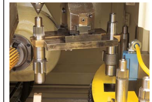
The Drake carousel system provides precise gear handling and smooth, consistent work flow for maximum productivity.
