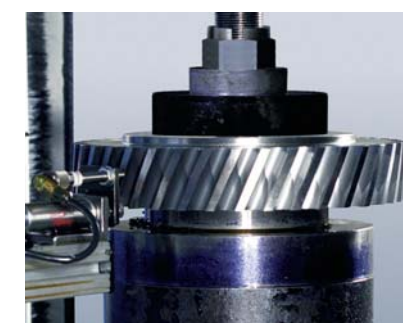
Stock divider automatically locates tooth position.
